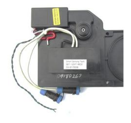
The **S2VT Pro-Series valves** have 2 white wires coming out of the module that connect to the switch(es) or extension cables. The replacement part number is **5878.**
