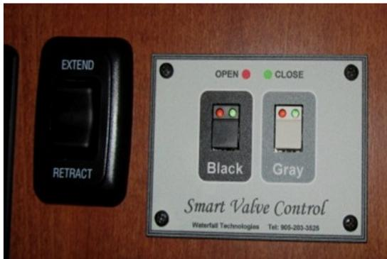
**Fig. 17 C** Double switch panel mounted (Note: no rear access after mounting)
